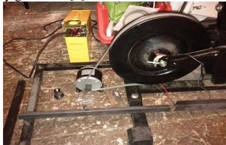
Figure 6: Belt Drive in Flywheel energy generation
